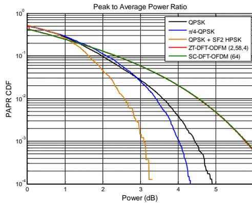
**Figure 2-5 PAPR of single carrier waveforms**
