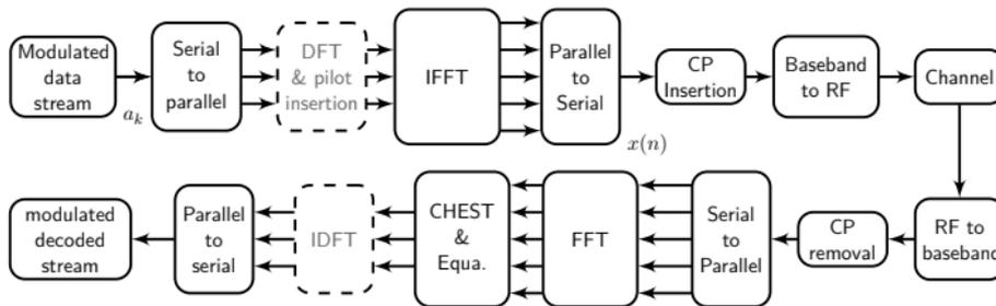
OFDM & SC-FDMA (additional stages in dash) transceiver scheme
