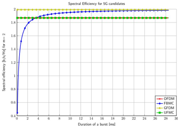
Comparison between SE of waveforms
