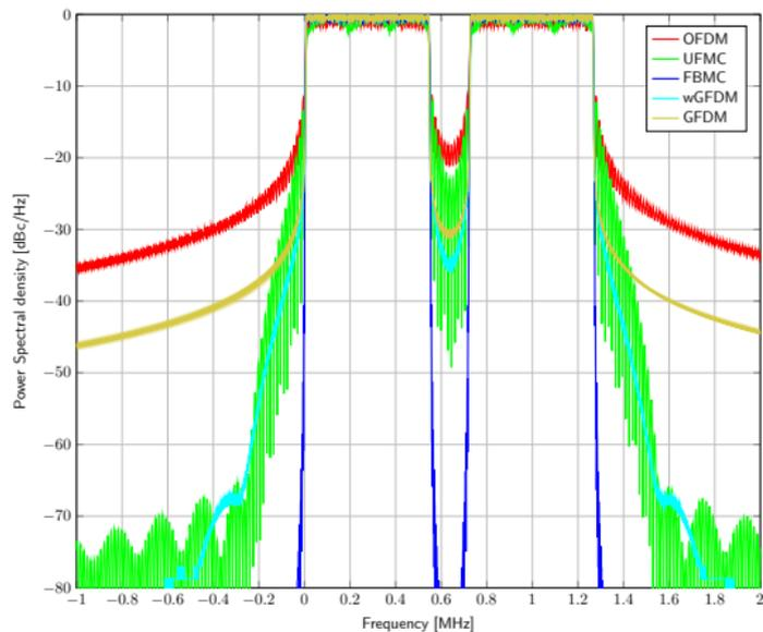
Power spectral density of waveforms
